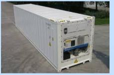
A refrigerated container is a shipping container used in intermodal freight transport that is refrigerated for the transportation of temperature sensitive cargo. Reefer containers usually have their own refrigeration unit, with an air or water cooled heat exchanger. They have their own data logger to record temperature.
